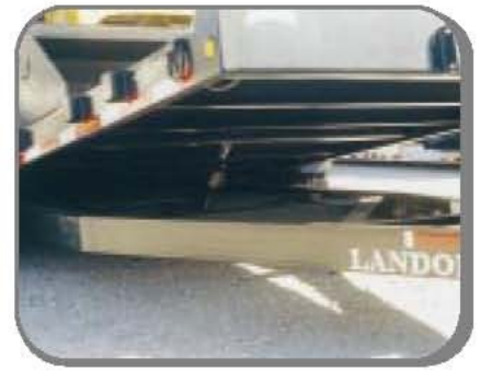
Landoll's tilt control system and the 2-1/2" x 16" cushion cylinder can hold the deck in a tilted position or smoothly return the deck to transport position.
