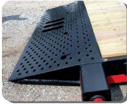
A full width rear light bar and Landoll traction plate makes loading small wheel machines efficient.
