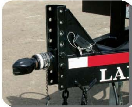
The hitch adjusts from 12" to 24" vertically.
