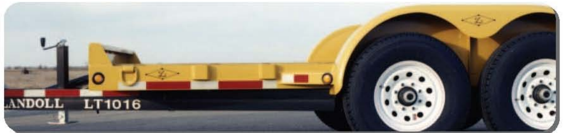
A 6"channel iron frame under the main frame for superior strength. A solid formed 6" height headboard for protection. (Stake pockets shown for optional removable sideboards.)
