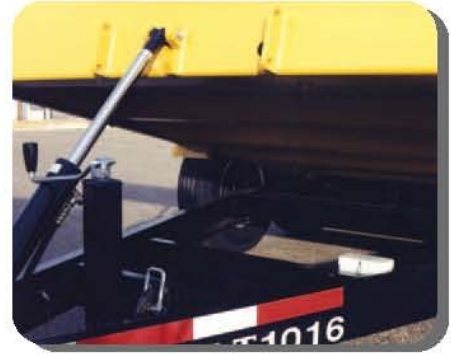
The cushion cylinders tilt the bed to ground load position and back to transport position smoothly.
