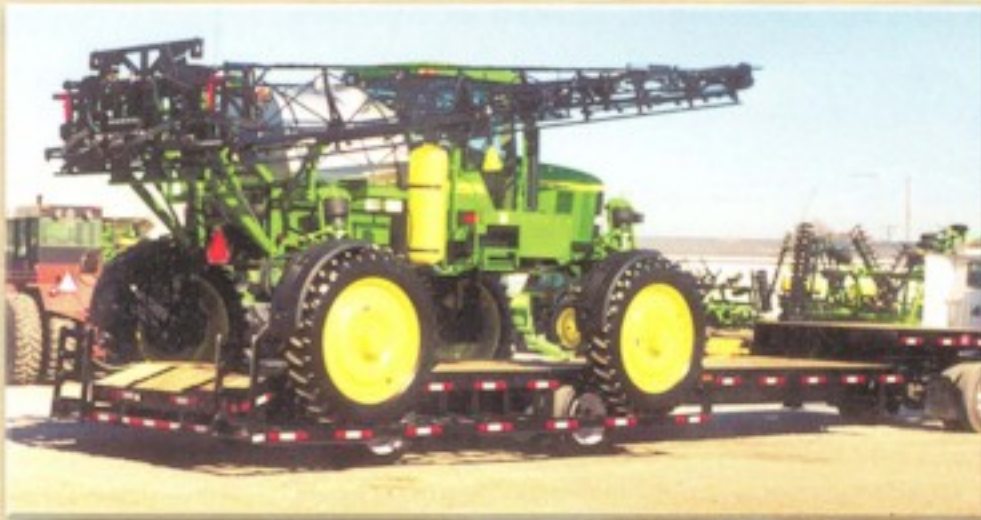
48' Sprayer Special Dropdeck with rear pull out extensions to haul high wheel sprayer
