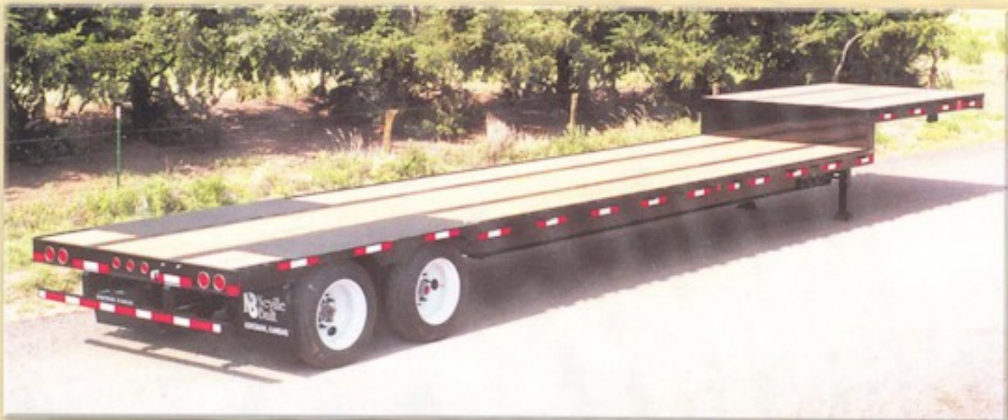
48' Dropdeck, no beavertail. We custom build flat frame & dropdeck chassis.
