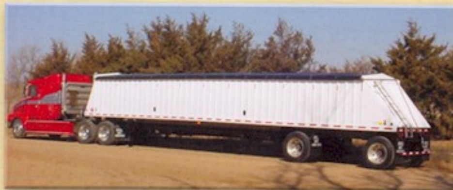
49' Vertical Rib - Double Hopper - Spread Axle Airride w/Aluminum Wheels
